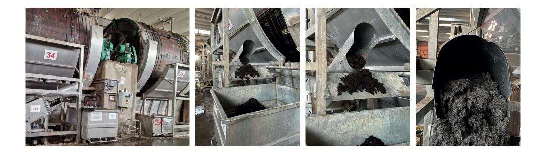
New system for separating hair from leathers, this optimization process allows us to use less water and fewer chemicals in the lime and tanning phase.
