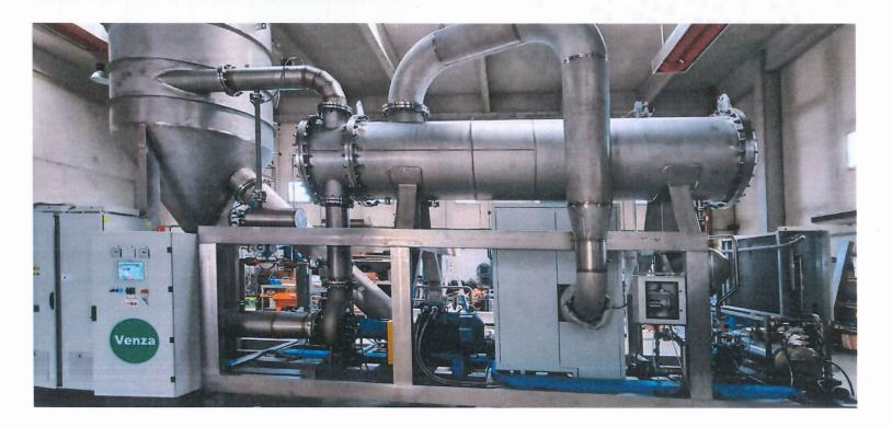
Together with the University of Padua, we have studied and implemented the prototype of the treatment of liquid finishing waste that allows us to reuse 97% of the water, while the solid residue, after being centrifuged, becomes usable material as fuel in blast furnaces to produce cement.
